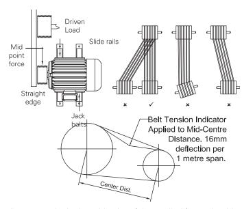
As a general rule the mid point of the applied force should be at the mid point of the shaft and it is good engineering practice to mount the motor pulley with hub and locking screw at the shaft end.
