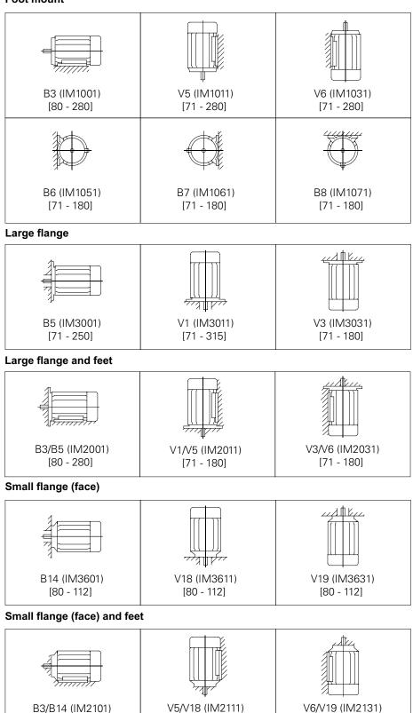
Note: Bearing arrangement may require review for vertical shaft mounting.
